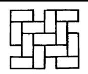
Bricks are 3%" x 7¾" with ½" mortar joints arranged in a herringbone pattern
