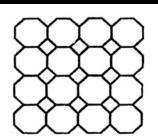
Octagonal tile 7¾" wide with ½" mortar joints interspersed with 3" diamond/square tiles Width: 33"
