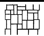
Random squares and rectangles ranging in size from 2¾" x 4¾" to 11" x 12" with mortar joints ranging from ½" to 1" wide Width: 36"
