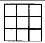
Tiles are 5½" square with 1/2" mortar joints arranged in a stacked bond pattern Width: 36"
