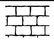
Bricks are 5½" x 9" with irregular/curved mortar joints arranged in a running bond pattern (simulates old or used brick) Width: 36"
