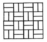
Bricks are 3%" x 7¾" with ½" mortar joints arranged in a basket weave pattern Width: 33"
