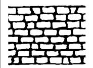
Random broken bricks ranging in size from 2½" x 3¾" to 3¾" x 9" with mortar joints ranging from ½" to 1½" Width: 37"
