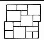
Random squares and rectangles ranging in size from 5" x 5" to 11" x 13½" with ¾" mortar joints Width: 36"
