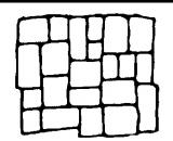
Random shaped stones with highly rounded corners ranging from 31/4" x 31/2" to 7" x 81/4" with irregular mortar ioints Width: 33"
