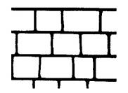
Random size stones ranging from 5" x 5" to 5" x 10" with ½" mortar joints, with rounded corners, straight longitudinal mortar joints and irregularly curved lateral mortar joints Width: 33"
