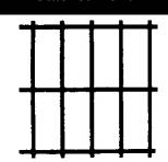
Bricks are 3.9" x 73/4" with ½" mortar joints arranged in a stacked bond pattern Width: 33"
